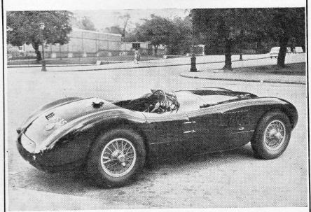
This "C Type," victor of many first-class events, has been greatly developed by the Ecurie Ecosse who modified the engine, brakes and suspension. It has lately been further improved by the addition of Weber 45 mm twin choke carburetters and the latest type head and camshafts. It has been completely overhauled by Jaguar Cars Ltd., and is immediately ready for racing. Panelling is finished in B.R.G. and is virtually unmarked. See "Autocar," 18/3/55, T.O.S.C.
