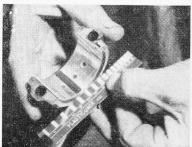
First dismantle the bearing and wipe away the oil. Break off a piece of the Plastigauge rod and lay it on the lower bearing half.
