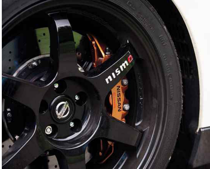
Above: 20in Rays alloys come complete with knurling to prevent the tyres from slipping around the wheels during heavy braking or acceleration
