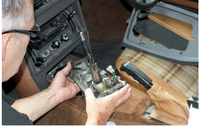
13 Taking care not to smear grease across that lovely light beige tartan interior, Simon could now lift out the remote linkage itself to see if that shed any light on the problem.
