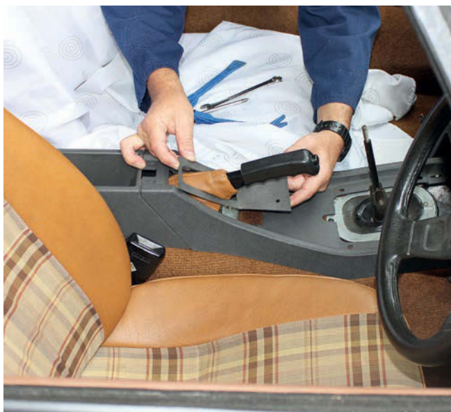
5 So did this plastic closing panel that went around the gear stick – it was a tight squeeze, but could be gently manoeuvred past the handle. Fortunately Triumph did not go in for multiple hidden fixings on the TR7.
