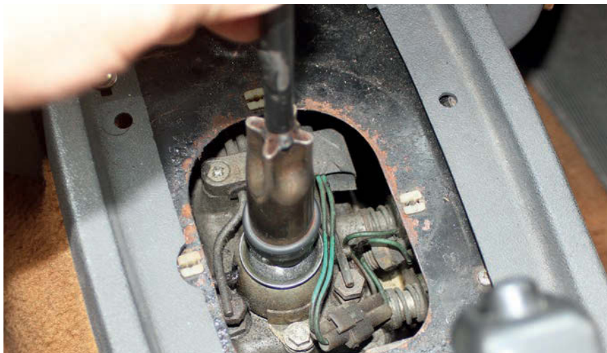
3 Simon was expecting to find play in the gear stick because the plastic cup underneath its ball had broken up or worn, but there was no movement there. However, the entire remote linkage did move from side to side.
