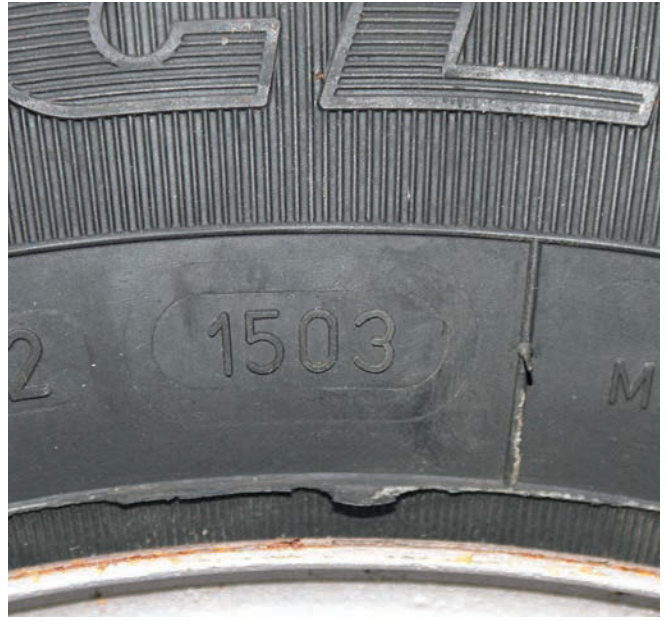
12 Unfortunately, this mark on the sidewall indicated that they had been manufactured in the 15th week of 2003 – at 19 years old, they had to be replaced.
