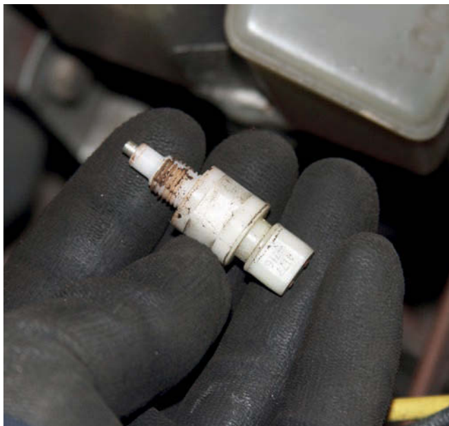
15 Bleeding the brakes produced a disappointing fluid flow, but referring to the manual showed that this brake pressure failure switch had to be removed from under the master cylinder before bleeding. You live and learn!
