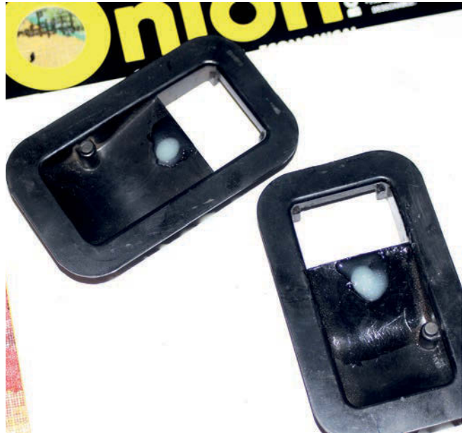
14 Rather than try to glue just the cracks together (previous owner Joh had already tried that), Simon filled the whole of the screw holes with epoxy resin.
