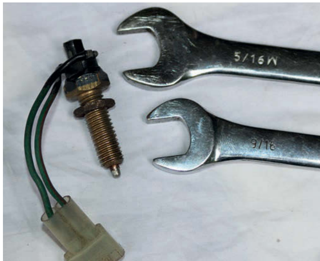
20 A NOS reverse light switch was also needed. This turned out to need a Whitworth spanner – you often find with instruments, carburettors and pipe fittings that spanners such as BA or Whitworth are required.
