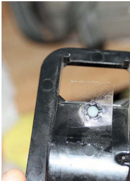
15 Putting a strip of Cellotape underneath stopped the glue leaking out before it had set and made the cracked plastic structurally sound.
