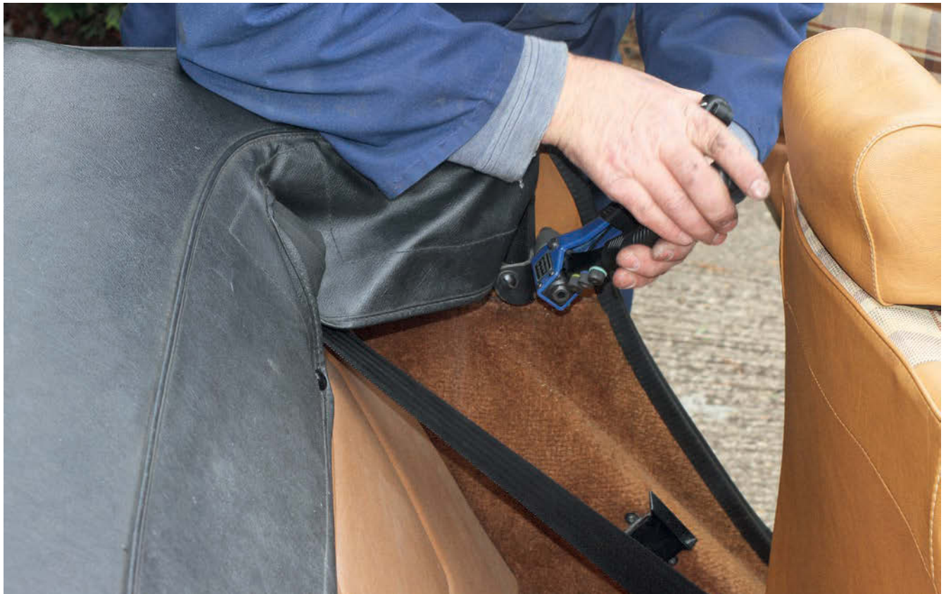
16 The answer for now was to rivet the fastenings directly to the B-posts. (The hood cover is not purely decorative, but stops the folded roof from billowing out when it is in the stowed position.)
