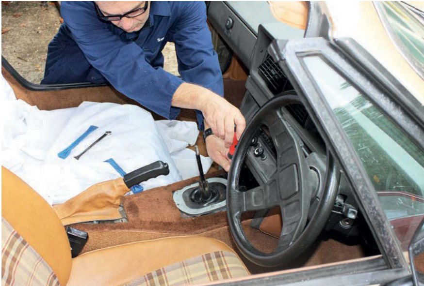
7 We still did not have access to the remote housing though, as first we had to remove this metal clamp that was screwed into the propshaft tunnel.
