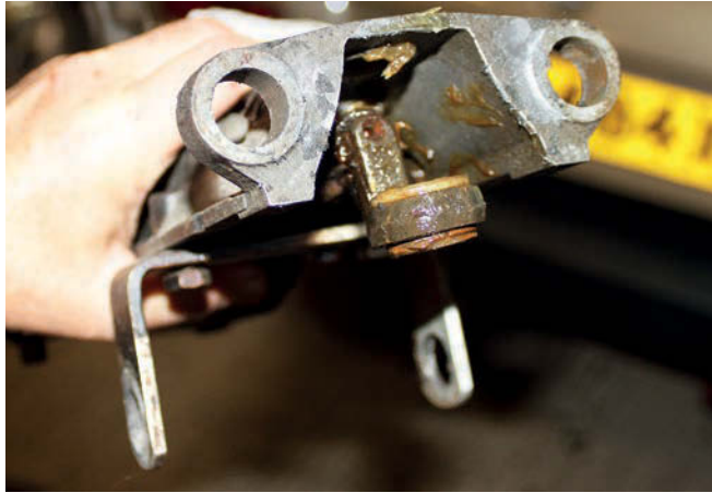
14 It made little sense at this point because the holes in the remote housing were so much bigger than the metal bushes on the bolt. Note too the swivel bush in the centre that sits on the end of the rod connected to the bottom of gear stick.
