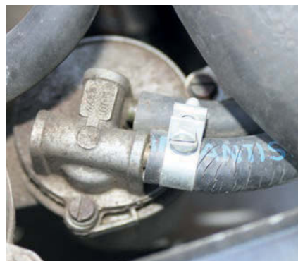
9 While messing about in the engine bay, Simon spotted something that he really should have noticed earlier – petrol pipes that were badly cracked.
