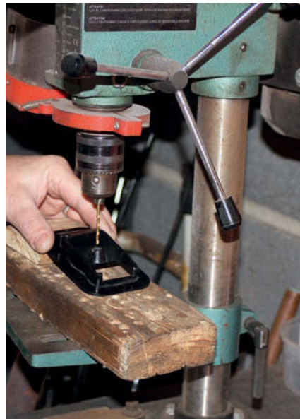
16 Holes for the fixing screw could then be drilled through the resin, and a chamfer for the countersunk head put into the top with a larger drill bit.
