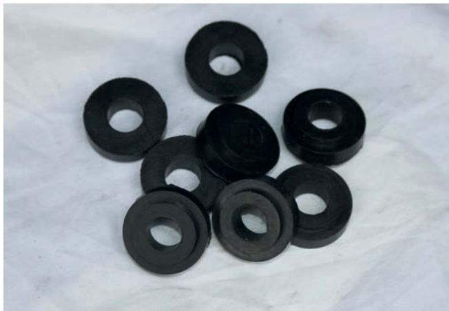
16 In the meantime, Simon had figured out where the problem lay – this set of eight top hat bushes were missing from the car. A new set cost £16.80.
