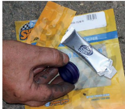
6 A SuperPro polyurethane bush for the bulkhead only cost £10.74, and came with its own sachet of silicone grease.
