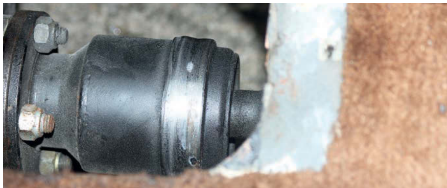
19 There were witness marks to this contact on the CV joint at the front of the propshaft. It did not look to have caused any permanent damage, but could this have contributed to a vibration through the seat at 60mph?
