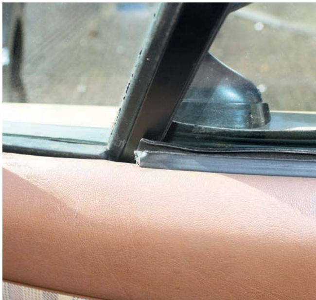
18 ...but on the driver's side, the interior weatherstrip did not appear to sit properly by the quarterlight glass.
