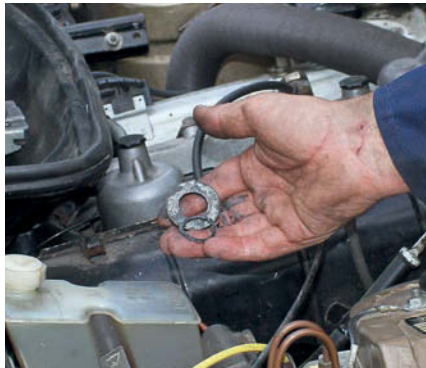
5 This was the washer that had made it difficult to see that the bush was missing and that was why the steering shaft was able to move about.
