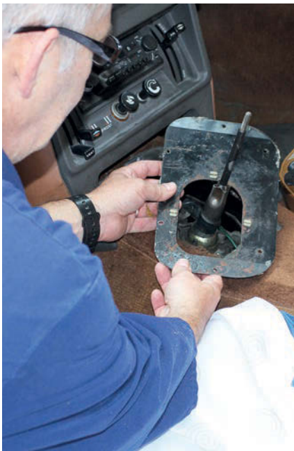
9 Finally, there was one more metal plate to remove and wiggle up through the opening cut into the carpet.
