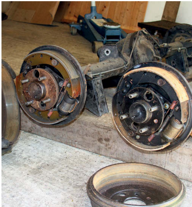
10 Because the wheel cylinders on the car had been filled with silicone fluid and the ones on the replacement axle probably had not, Simon transferred everything from the original axle across to the new one.
