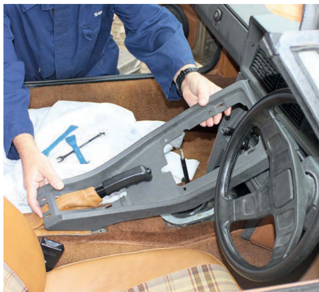
6 After searching out any remaining screws holding on the central cubby between the seats, that could be removed. It was followed by this section that went around the handbrake lever and the gearstick.
