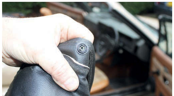
18 Forcing then on was not made any easier by the fact that the poppers were plastic – get the angle slightly wrong and the plastic would deform and never go on. Simon does have a cunning plan for the hood cover, though!
