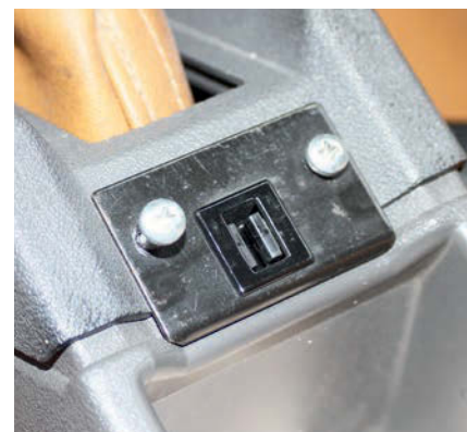
4 Needing better access to investigate this problem, the plastic centre console had to come out. There is not always a set order in which pieces have to come off, but this clip had to be removed to separate the two halves of the console.
