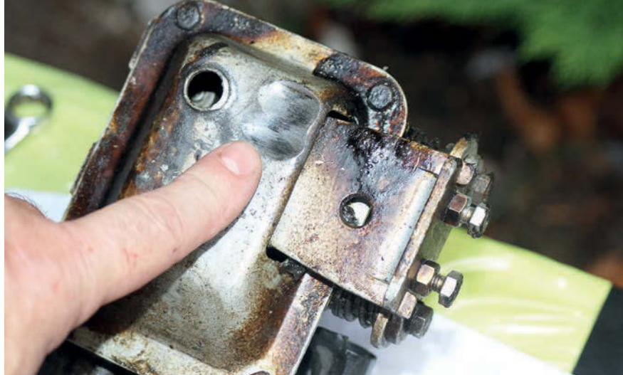
18 Without the bushes, the linkage had been able to move about to the extent that it could foul on the joint at the front end of the propshaft situated just below it. That would explain the grinding noise.
