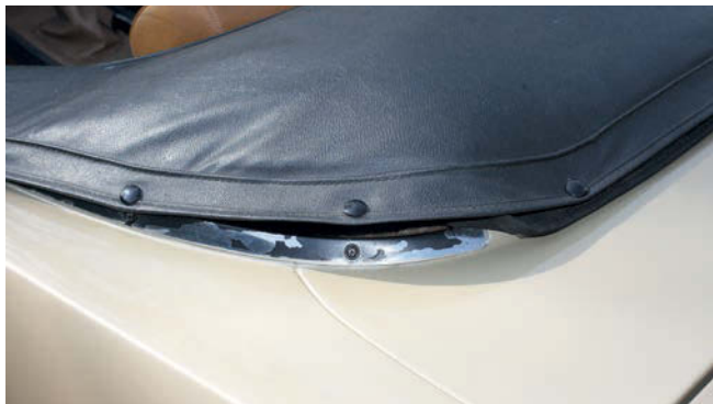
17 Unfortunately, moving the hood frame did not make it any easier to stretch the vinyl hood cover over the folded mohair fabric, and invariably one or two poppers had to be left unattached.
