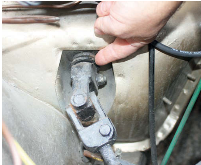
21 Pushing the car about on the drive also revealed another bush that was missing – one that should go here where the steering column passes through the bulkhead. Without it, the column was able to flex more than it should.
