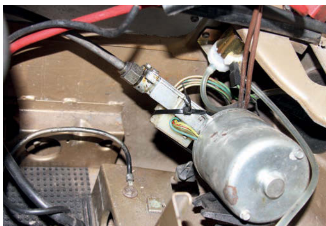
3 It was difficult to get in there and tighten it up fully though, so he added a cable tie to stop it moving back away from the motor, unaware that the problem was the loose screw, not the position of the motor.
