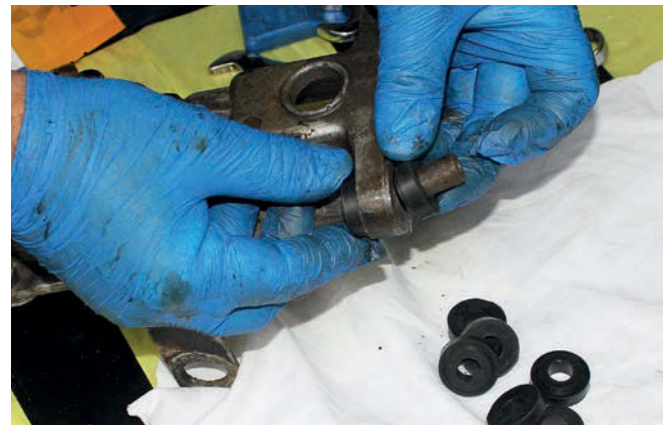
17 And this is where they should go – one either side of each hole in the remote linkage housing, with the steel bushes through the middle. That way, the holes were filled and the bushes protected from being crushed.
