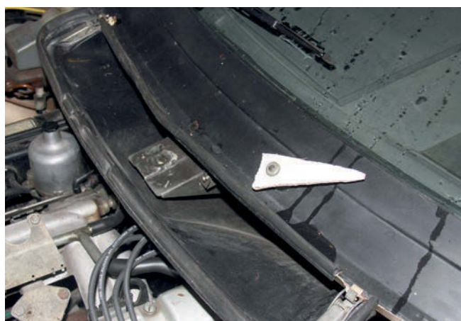
4 Eventually realising his mistake, the cable tie was removed, the wiper motor clamp removed and the wiper turned over and the screw done up tightly. A cardboard arrow instead of the wiper arms allowed for safe testing of the new parking position.
