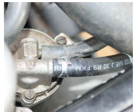
10 So he replaced all rubber fuel pipes with new hose rated as R9, which should be safe for use with today's ethanol-infused petrol.
