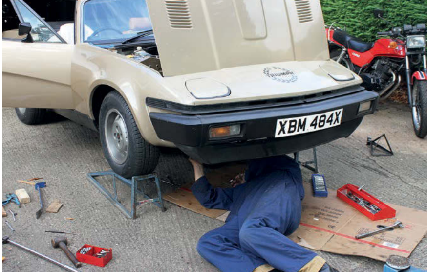
3 The pinch bolts securing the UJs to the shafts were easy enough to remove, but to create enough slack in the system to slide them off the splines, Simon undid the steering rack mounts and moved the rack forwards.
