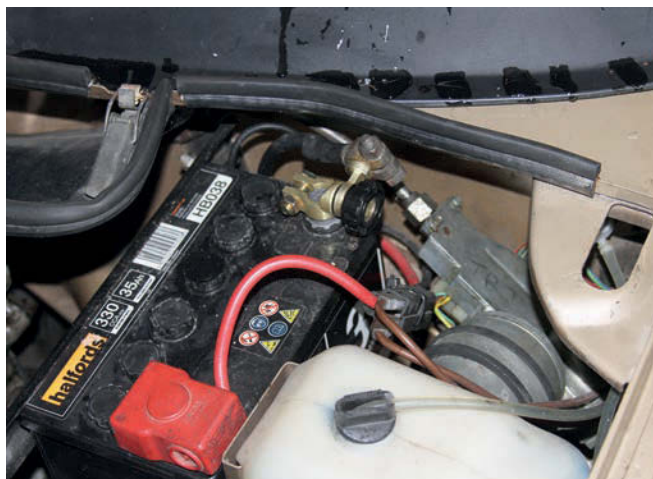
1 The wiper motor is tucked up on the nearside where the front inner wing meets the bulkhead. This one has the legend 'TR7' handwritten on it, suggesting that it is a secondhand replacement from a scrapyards or autojumble.
