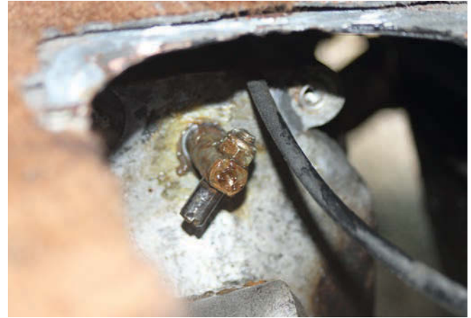
15 That swivel bush has to hook over this pin on the gear selection rod coming out of the gearbox in order to transfer your input at the stick to the cogs in the box. Keeping these two connected made reconnecting the linkage tricky in the confined space.
