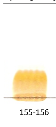
Fig. (17): TLC plate of compound AL-7 using system CH 2 Cl 2 / MeOH (75:25)
