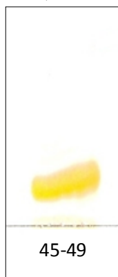
Fig. (18): TLC plate of compound AL-8 using system CH 2 Cl 2 / MeOH (80:20)
