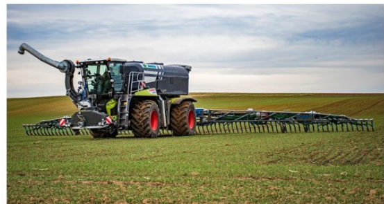
The 16 cubic metre Bauer PT17 poly tank and front-mounted filling pump system converts the Xerion 4000 S-Trac into a self-propelled slurry and digestate applicator.
