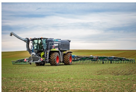
The 16m 3 Bauer PT17 poly tank and front-mounted filling pump system converts the Claas Xerion 4000 S-Trac into a self-propelled slurry and digestate applicator.
