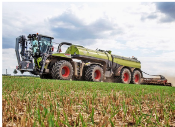
A 30,000-litre capacity semi-trailed slurry/digestate tanker on a Xerion 4000 S-Trac with front-mounted filling system
