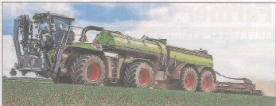
SPREADING GIANT A 30,000-litre capacity, semi-trailed slurry/digestate tanker on a Xerion 4000 S-Trac, fitted with a front-mounted filling system – that's a whole lot of slurry in one go!
