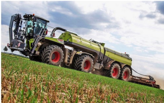
A 30,000-litre capacity semi-trailed slurry/digestate tanker on a Xerion 4000 S-Trac with front-mounted filling system.
