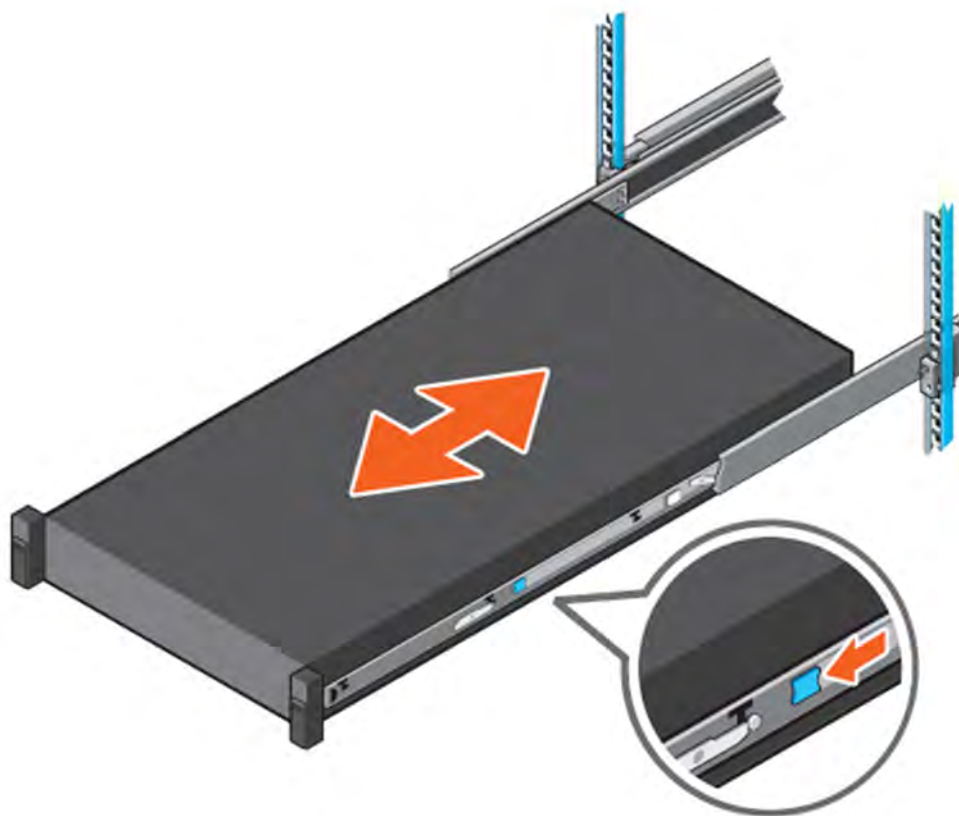
Figure 20. Slide system into the rack
