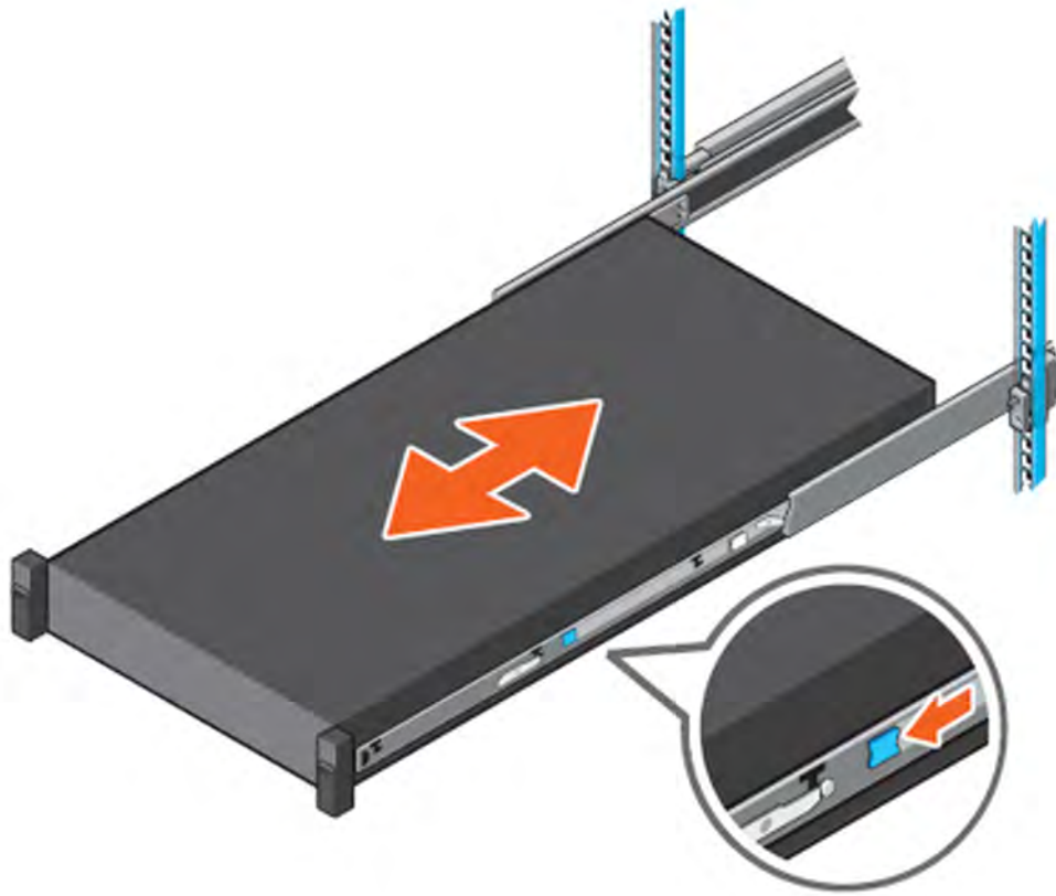
Figure 24. Slide system into the rack
