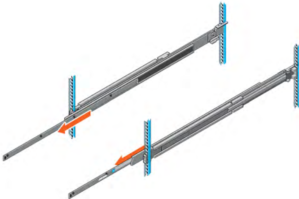
Figure 18. Pull out inner rail
