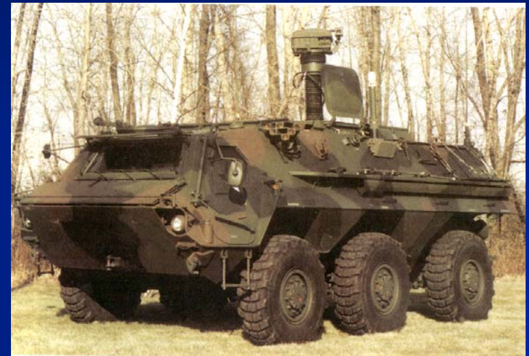
M93A1 FOX Reconnaissance System Nuclear and Chemical detection and Biological sampling
