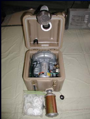
Dry Filter Unit (DFU)
