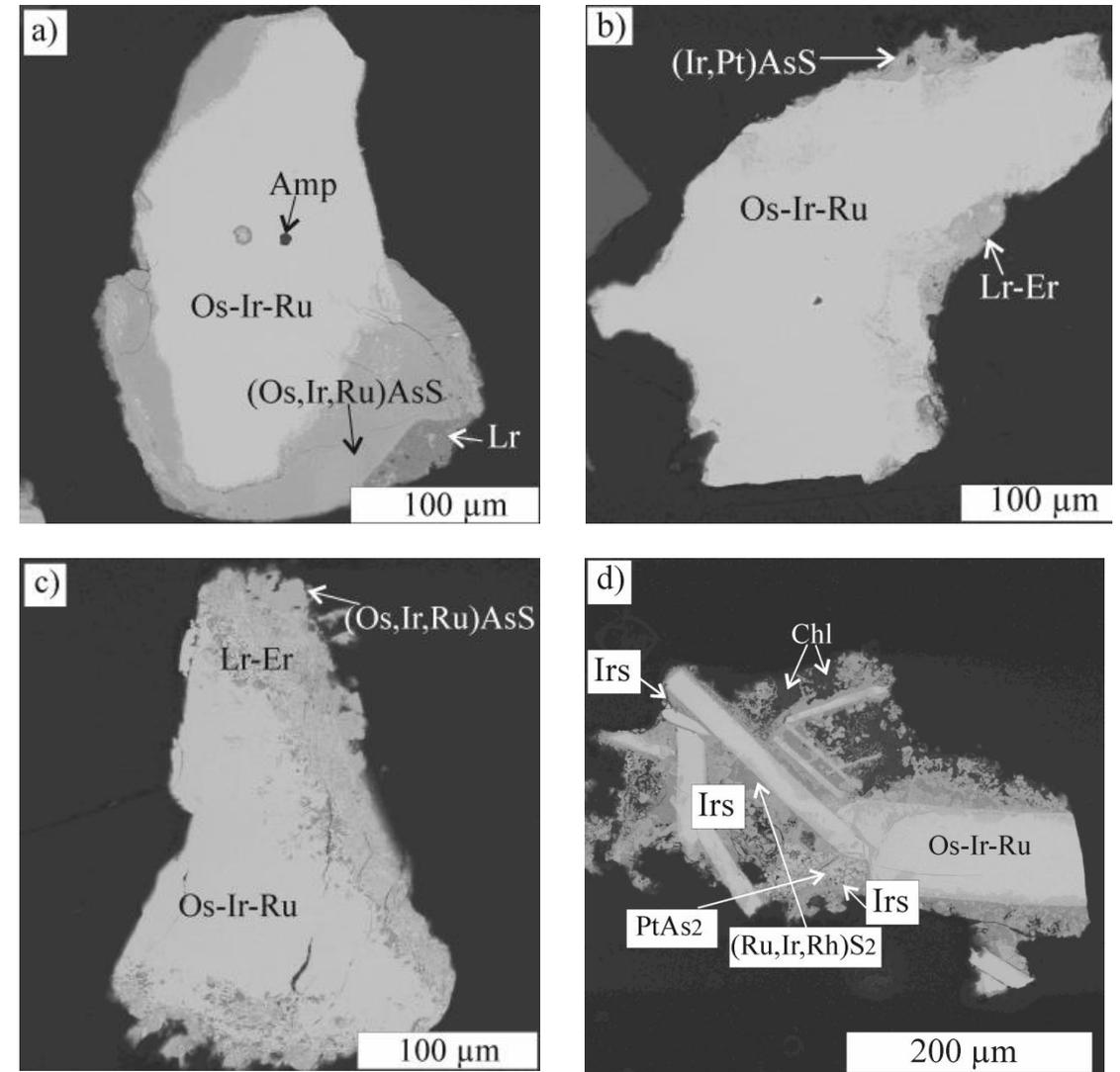
Figure 8. BSE images the platinum group minerals from the Kitoy alluvial placer
