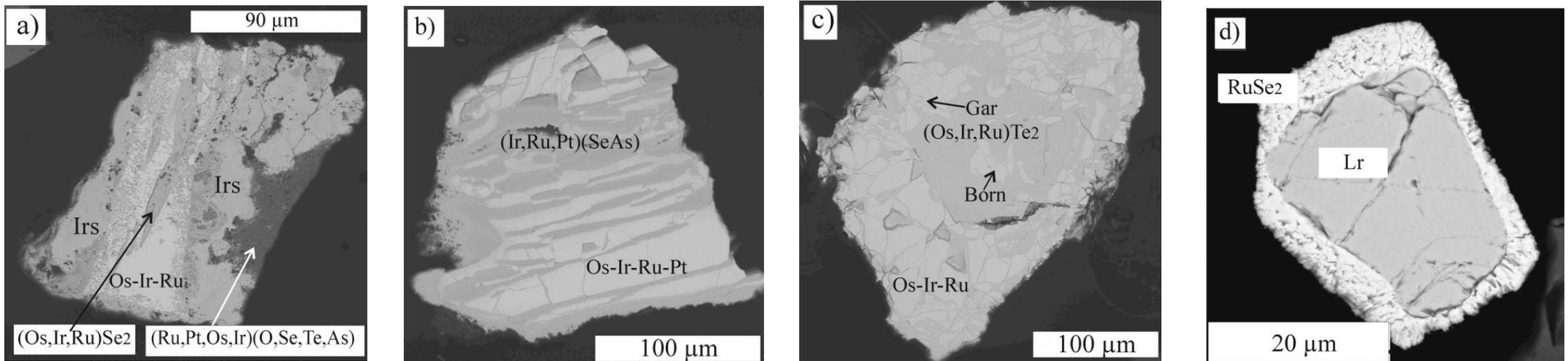
Figure 12. BSE images Se-, Te-ferrous platinum group minerals: a-c) from the Kitoy alluvial placer; d) from the chromitites of Dunzhugur ophiolite massif
