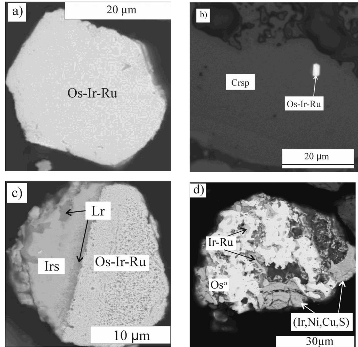
Figure 6. BSE images of the platinum group minerals (a, b) from chromitites of the south branch ophiolite; (c, d) from chromitites of the north branch ophiolite
