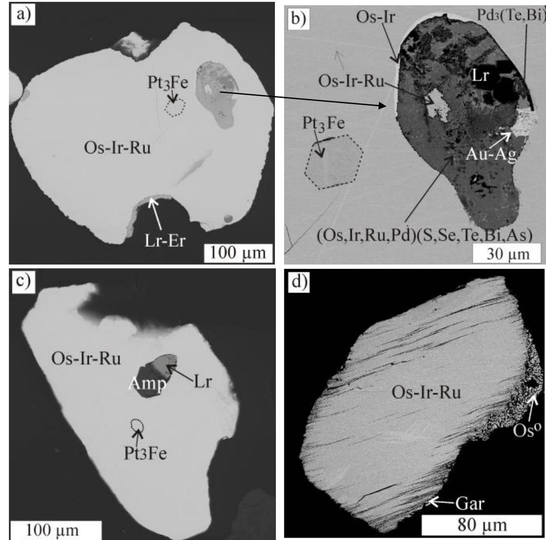
Figure 4. BSE images of the platinum group minerals from the Kitoy alluvial placer
