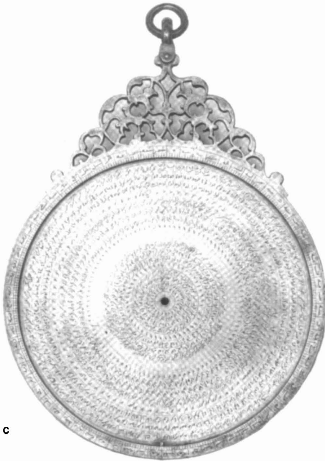
FIG. 2.6. AN ASTROLABE MADE IN 1060/1650 BY \text{ḌIYĀ}^{\text{P}} AL- \text{DĪN} MUḤAMMAD. Made in Lahore, in modern Pakistan, the parts of this astrolabe are: (a) rete; (b) plate for latitude 29^{\circ}\text{N} ; (c) mater or base; (d) back of the astrolabe.
