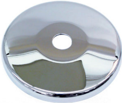
19" Single Disc Front Wheel Hubcap 4-3/4" chromed steel front wheel hubcap will fit all single disc 19" cast wheels on models with 9-spoke mag wheels from 1984-on. Replaces standard wheel hub plate and screws, and is held stationary between the front wheel hub's external bearing spacer and the front axle. 800 44467-88T
