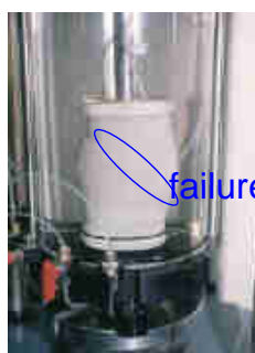
soil sample at failure
