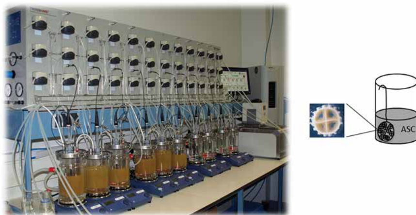
Fig. 1: TWINSHIME setup, consisting of two parallel SHIME systems. Each SHIME reactor contains 5 vessels simulating respectively the stomach, small intestine, ascending colon, transverse colon and descending colon. In each vessel of the M-SHIME (here the ascending colon is reported as an example) the mucosal compartment is formed by the addition of plastic microcosms (9 mm of diameter) coated with mucin type II-agar.
