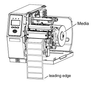
Route the Media counterclockwise, under and around the Rewinder Hub.
