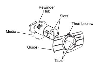
When it's time to unload the Internal Rewind option, tear or cut the Media (and, if installed, remove the Guide) then grasp and slide the Roll off the Rewinder Hub.
