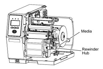
4) Insert the creased edge of the Media into a Slot, and then proceed according to the width:
