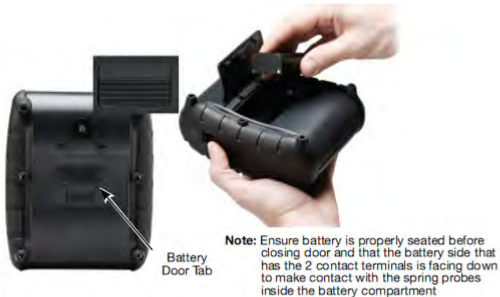
FIGURE 2: INSTALLING THE BATTERY CARTRIDGE
