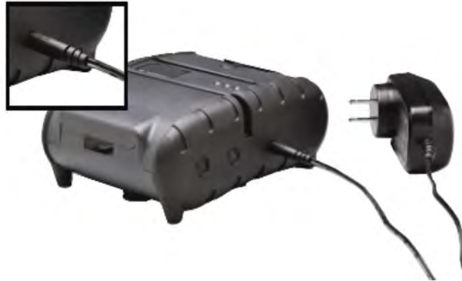
FIGURE 3: CHARGING THE BATTERY CARTRIDGE
