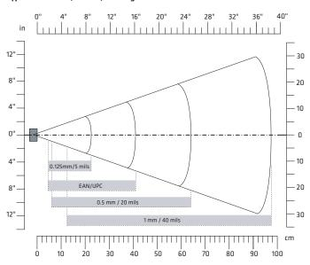
\*VESTA is an Intermec-patented algorithm that increases read range of Code 39 and EAN/UPC marks by an average of 60 percent (compared to EA31 read range with VESTA disabled).
