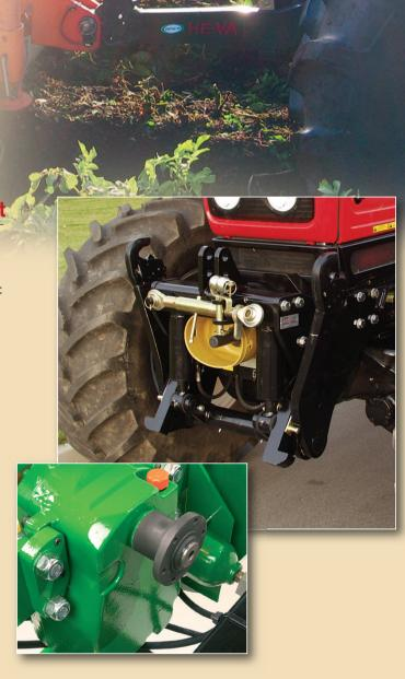
OPICO PTO's can be fitted to most linkages from 1.5 to 5.5 ton lift capacity.
