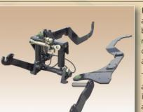
Fitting is simple and quick as the whole side plate can be removed. Also on most models, the linkage bolts onto the front of the tractor as well as the side.
