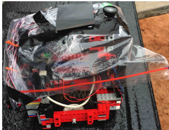
Figure 4.2: Robot doesn't like rain – the robot was successfully made water-resistant to mild rain with a plastic bag and electrical tape.
