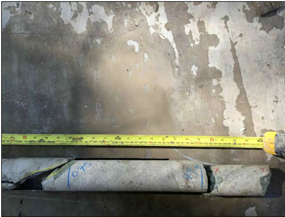
PHOTO 8: RHYOLITE ENCOUNTERED BELOW 46.30 m IN BH-BGC20-CW5-02.
