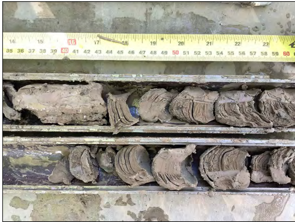
PHOTO 7: RHYTHMIC LAMINATIONS ENCOUNTERED WITHIN GLACIAL SEDIMENTS FROM 24 m TO 33 m IN BH-BGC20-CW5-02.
