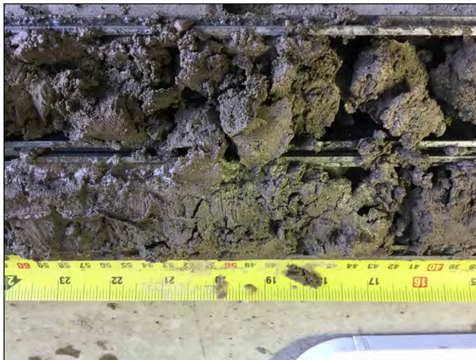
PHOTO 5: BH-BGC19-CW5-03 SPT 08 FROM 13.41 m TO 13.72 m IN TILL SAMPLE.
