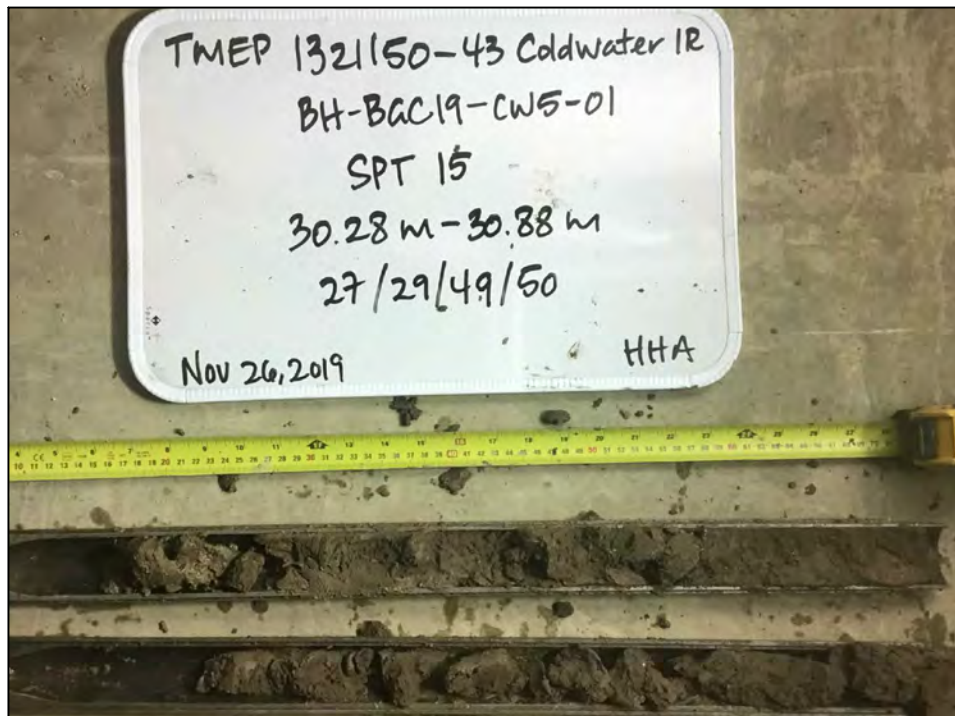
PHOTO 4: BH-BGC19-CW5-01 SPT 15 SAMPLE FROM 30.28 m TO 30.88 m. TYPICAL SAMPLE OF TILL FOUND IN BH-BGC20-CW19-CW5-01, BH-BGC19-CW5-03 AND BH-BGC20-CW5-02.
