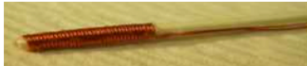
Figure 1. Solenoidal coil-tipped catheter, 30 AWG copper wire
