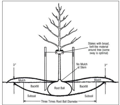
Figure 27. General hardware guidelines for tree installation
