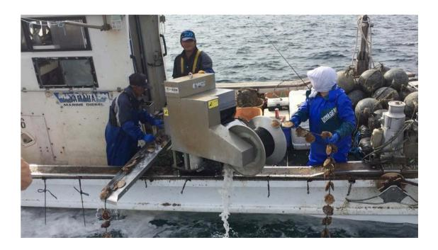
The machine positions scallops to lay flat and forces pressurized seawater onto the top and bottom shell surfaces of the scallops to remove algal growth and tunicates (think car wash). The scallops remain attached the vertical grow out line as it is fed through the cleaning machine and are deployed right back into the water after cleaning. Biofouling will vary by location and the need for repeat cleaning will also depend on local conditions.
