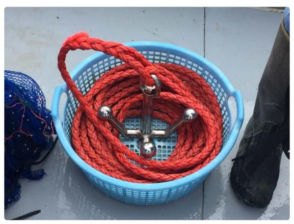
Grappling Hook used to secure long line to vessel Photo Credit: Hugh Cowperthwaite
