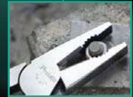
Screw/unscrew specially for stripped thread
