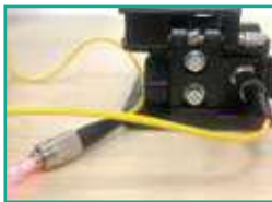
Visual Fault Locator Output Power: 1mW
