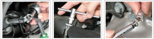
Universal joint Spinner T handle Extension bar w/2 way
