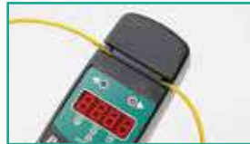
Identify 270Hz, 1KHz, 2KHz with buzzer indication
