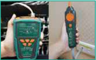
Verify LAN/ telephone cable condition
