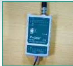
BNC cable test
