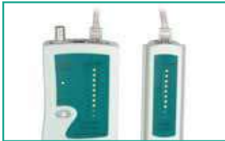
Pin to pin cable mapping
