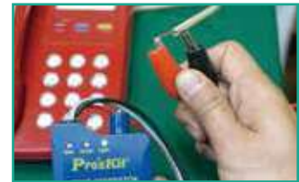
Phone line polarity indication and status check
