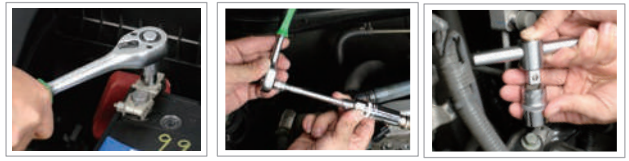
Teeth reverse flat ratchet handle Spark plug socket Sliding T handle with quick release
