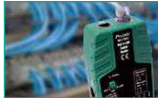
Live Ethernet cable test
