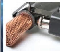
Cable slitting and stripping
