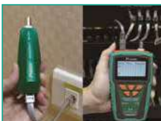
Verify LAN / Telephone / Coaxial cable condition
