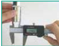
Inside dimension measurement
