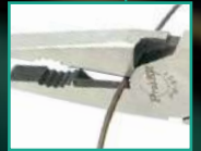
Cutting capability for 2.0mm Piano wire
