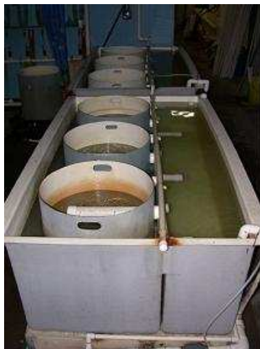
Upwell/downwell system used for setting pediveligers
