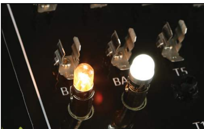
Standard bulb vs. Bulb style LED MATT
