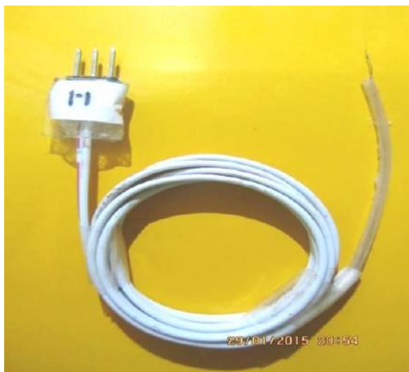
Figure 1. Thermocouple instrument for measuring the temperature used during the study
