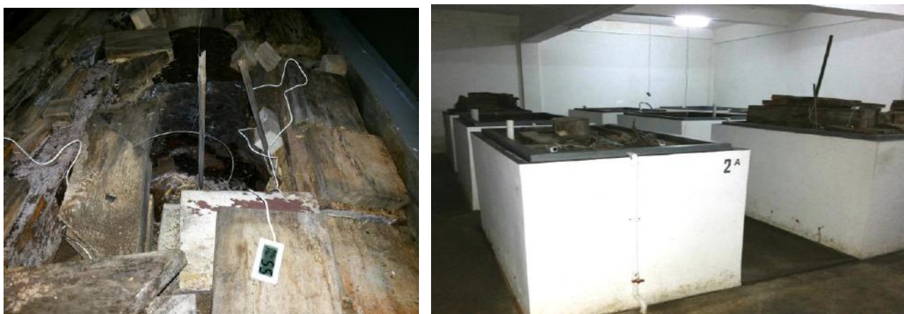
Figure 2. Thermocouples were laid in Coptotermes curvignathus rearing chambers in the Termite Laboratory
