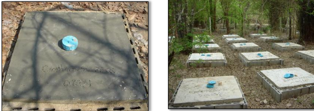
Figure 2 Plot of termiticides test by Modified Ground Board (MBG).
