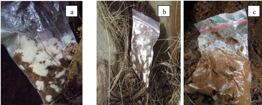
Figure 4. Condition of Copton 0.5 RB termite bait with 0.5% hexaflumuron bait at 7 days after installation (a), 14 days after installation (b) and 21 days after installation (c)
