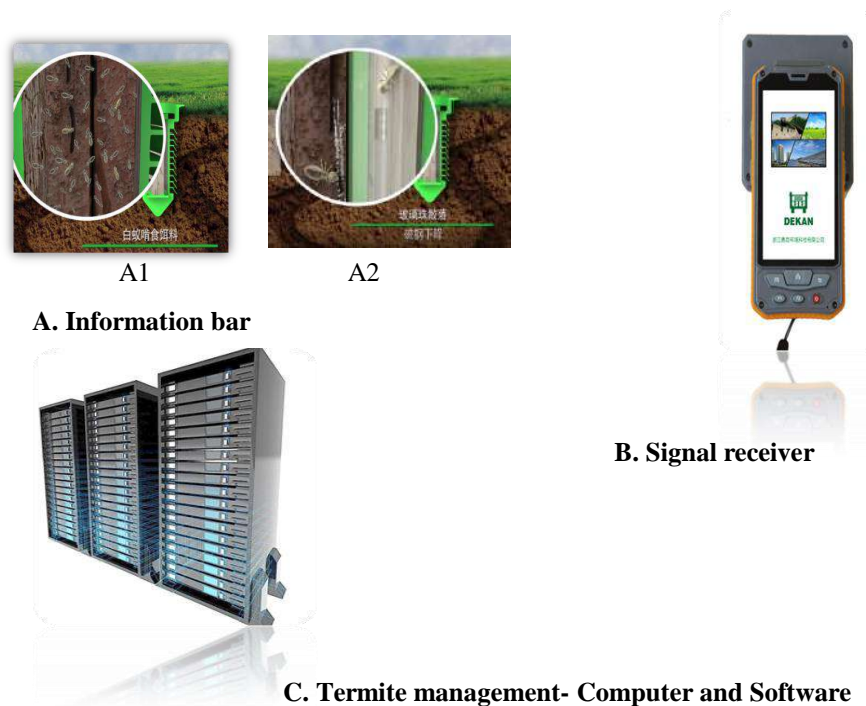
Figure 1. The components of a device with non-looping electromagnetic induction for remote monitoring of termites. The device consists of three parts, A. Information Bar. B. Signal Receiver. C. Termite Management Computer and Software. A1: The situation when termites consume the information bar. A2. The spherical particulate within the information bar and the permanent magnet. The magnet drops while the information bar is consumed by termites.
