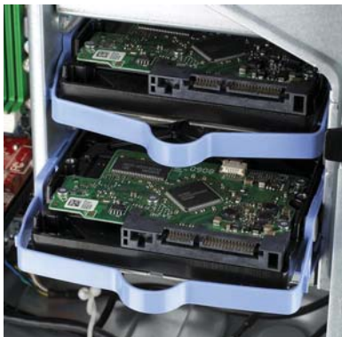
Lenovo IdeaCentre K300 toolless disk drive removal
