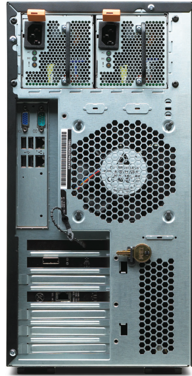
Lenovo ThinkServer TS200 with Redundant Power Supply
