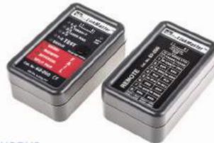
328-7856 Ideal Linkmaster Video, Data & Voice Wiring Tester of Cable Continuity, Miswire, Open Circuit, Short Circuit 62-200
