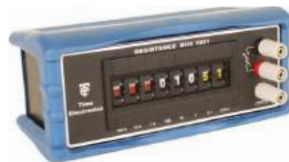
610-297 Time Electronic 1051 Decade Box, Decade Box Type Resistance, Resistance Resolution 0.01Ω 1051
