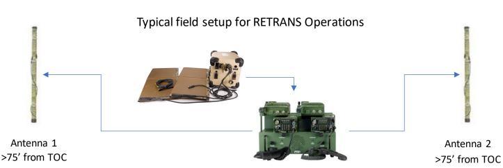
TOC Area Power Source & PSDS connected with 100' LMR400 feedline (CAB.OTH.101)
