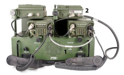
AS0004-SR-SR4A shown with unit supplied radios and cables populated. 1. AS0004-RTC RETRANS Cable, 2. Feedline and PA jumpers
