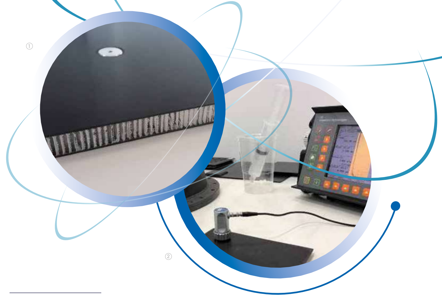
[1] Example of a CFRP sandwich panel manufactured at OPTIMAL [2] Quality control - ultrasonic inspection [Phased Array], composites and metallics
