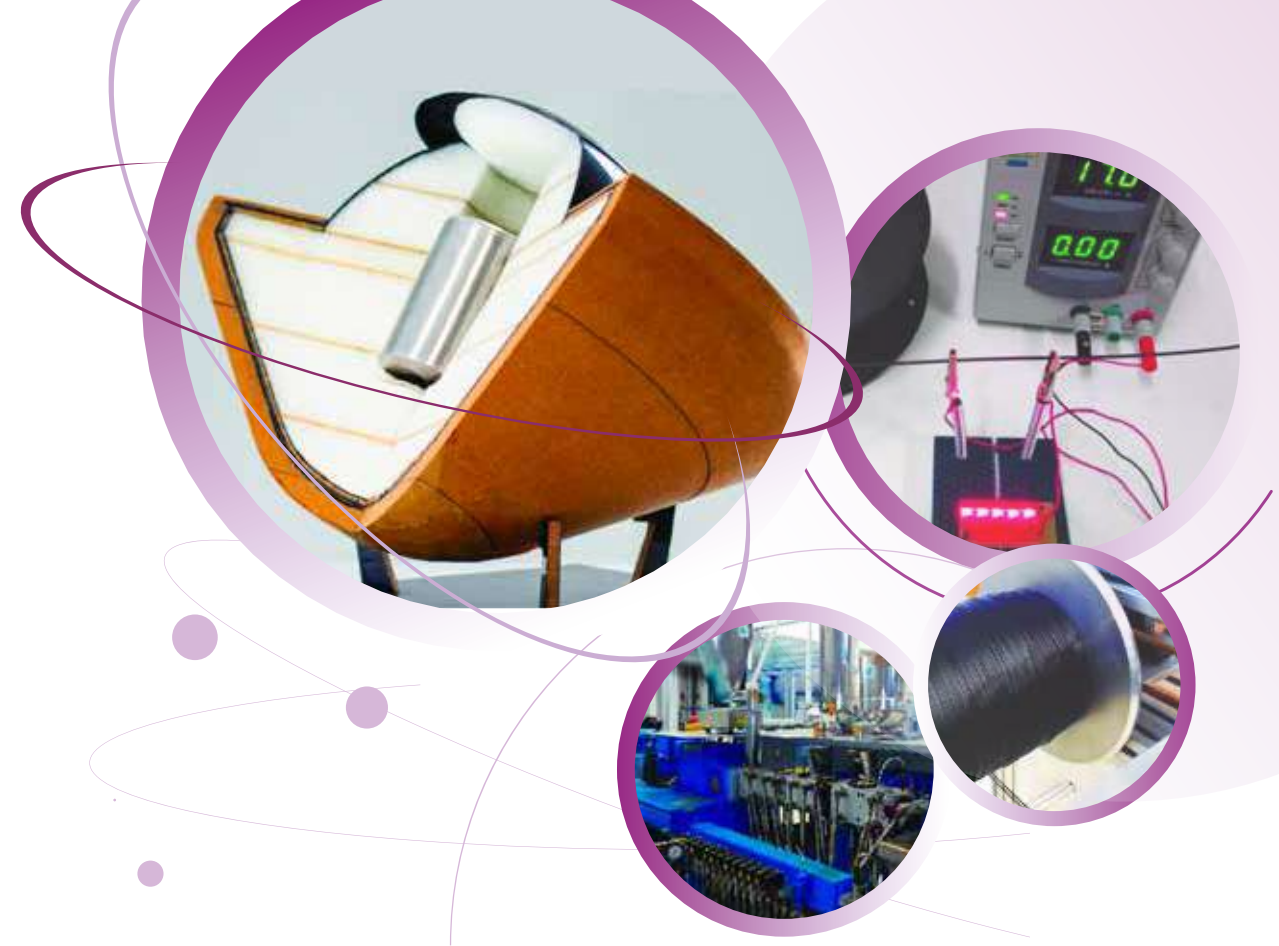
[1] ESA CTPS Breadboard after tested and sliced to view results [2+3+4] Production setup and test of the filament produced
