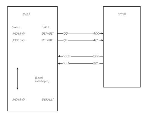
Note: In this example, UNDESIG refers collectively to all groups not assigned to a transport class. In this case, every group on the system uses the signalling resources assigned to the transport class DEFAULT.
