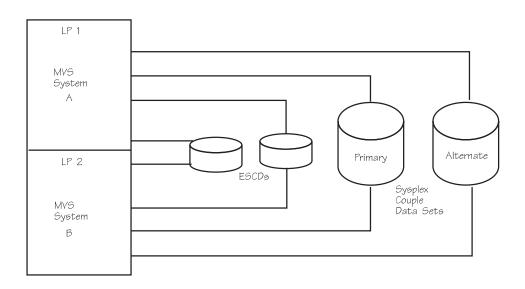
Figure 72. On PR/SM - Physical Configuration of a Sysplex on LPARs
