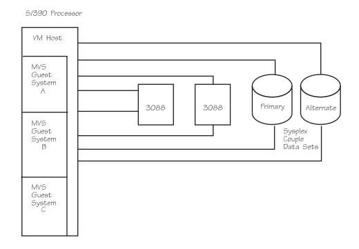
Figure 71. Under VM - Physical Configuration of a Sysplex With MVS Guests
