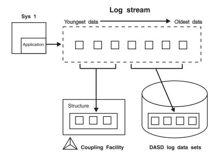
Figure 46. Log Stream Data on the Coupling Facility and DASD
