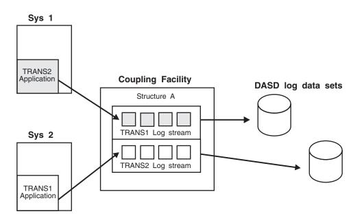
Figure 51. Example: Maintaining Multiple Log Streams in the Same Coupling Facility Structure
