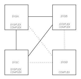
The dotted lines represent existing connections between the systems in the global resource serialization complex.
