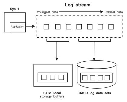
Figure 47. Log Stream Data in Local Storage Buffers and DASD Log Data Sets
