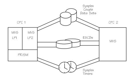
Figure 73. Configuration of a Sysplex on LPAR and Non-LPAR Systems
