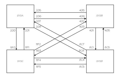
Figure 3. Signaling on a Four-System Sysplex, Implemented through CTC Connections
