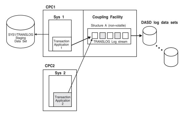
Figure 54. Example: Using Staging Data Sets When the Coupling Facility Shares a CPC with a System
