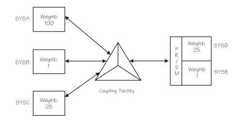
Figure 37. Failure Management with SFM Policy and a Coupling Facility
