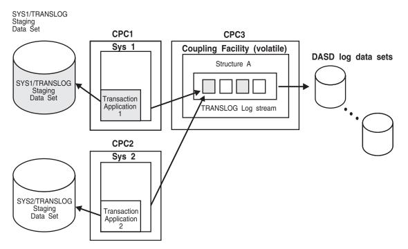
Figure 55. Example: Using Staging Data Sets When the Coupling Facility is Volatile
