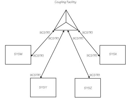
Figure 5. Signaling on a Four-System Sysplex, Implemented through a Coupling Facility List Structure
