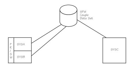
Figure 33. Three-System Sysplex on Two Processors with Active SFM Policy
