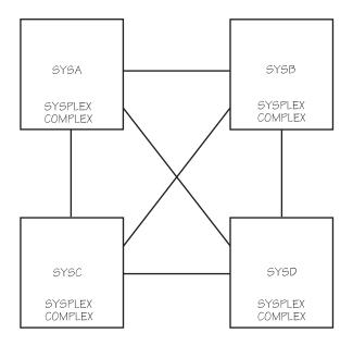
The lines represent the signalling paths between the systems.
