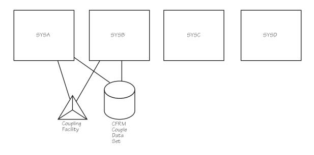
Figure 45. Multisystem Sysplex Configuration with a Coupling Facility
