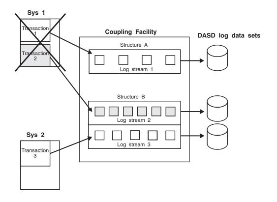
Figure 53. Example: Recovery for a Failing System - Recovery Delayed for Some Data
