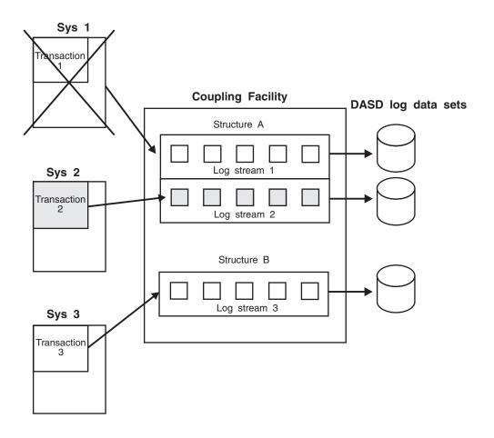
Figure 52. Example: Recovery for a Failing System - All Data Recovered
