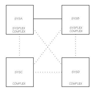
The dotted lines represent existing connections between the systems in the global resource serialization complex.
