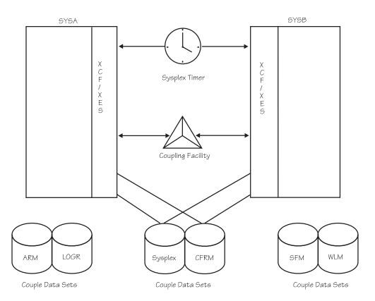
Figure 1. Sysplex with Coupling Facility and Couple Data Sets
