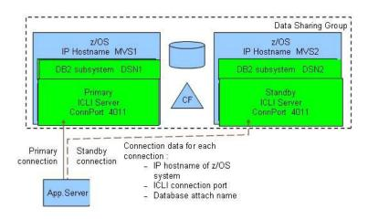
Figure 7. Option 0: Single DB2 member with passive (inactive) standby member
