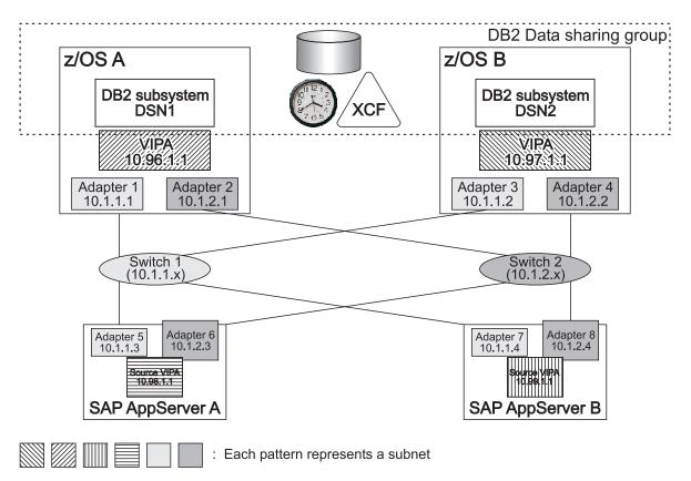
Figure 18. Recommended setup for a high availability network
