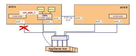
Figure 26. Rerouting if a network adapter card fails
