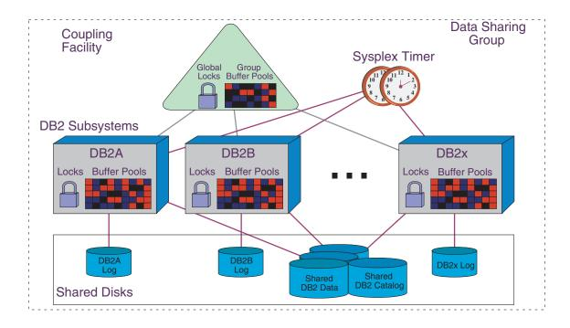
Figure 5. DB2 data sharing in a Parallel Sysplex
