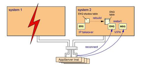
Figure 22. Failure of SCS and recovery of the enqueue table
