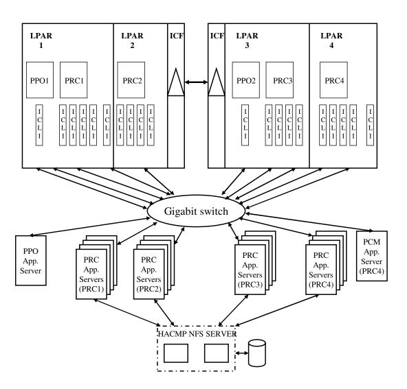
Figure 9. Large company using architecture options 0 and 1
