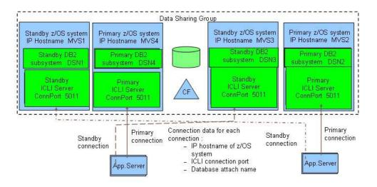
Figure 11. Option 3: Two active DB2 members, each with a passive standby member in an independent LPAR
