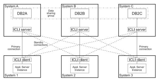
Figure 31. Application servers connected to primary and standby database servers
