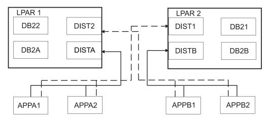
Figure 32. Failover setup using DB2 Connect, with multiple DB2 members in the same LPAR
