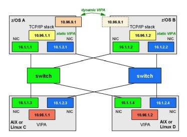
Figure 24. General concept of a fault-tolerant network
