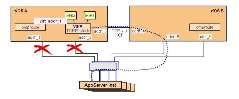
Figure 27. Rerouting in a sysplex even in case of two failing network cards
