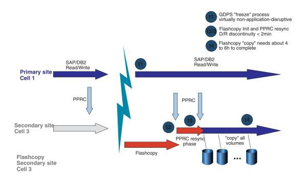
Figure 14. Process for obtaining a non-disruptive volume backup without the BACKUP SYSTEM utility of DB2 V8
