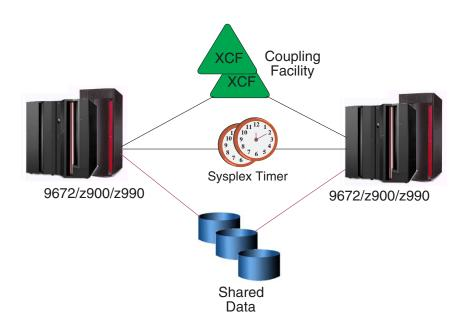
Figure 4. zSeries Parallel Sysplex architecture elements
