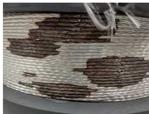
Figure 4.1.12. Coil made by OI and heat treated at the ASC. Surprisingly, the coil showed significant leakage.
