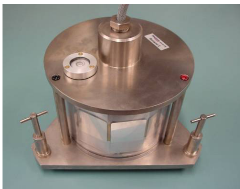
Figure 1a –Temperature stabilized sensor accommodated in a well isolated tripod for field applications.
