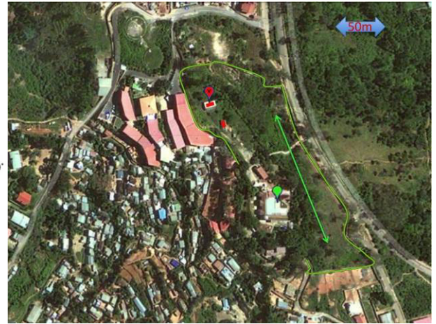
Figure 3 –Historical site of the TAN magnetic observatory nearby the University. Red: Variometer house ("V") and absolute measurements' hut; Green arrow: main electric power line; Green curve: wall of the IOGA institute that underline the "protected area" around the observatory.
