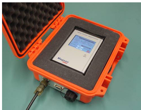
Figure 1b –Digital fluxgate electronics with touch screen and WEB interface. Can be thermally controlled as well.
