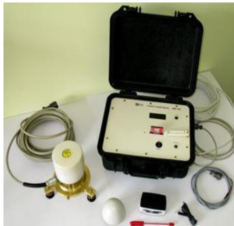
Figure 1 –The 1-sec Fluxgate Magnetometer LEMI-025. Figure adopted from the website of the Lviv Centre of Institute of Space Research (Korepanov, 2010).
