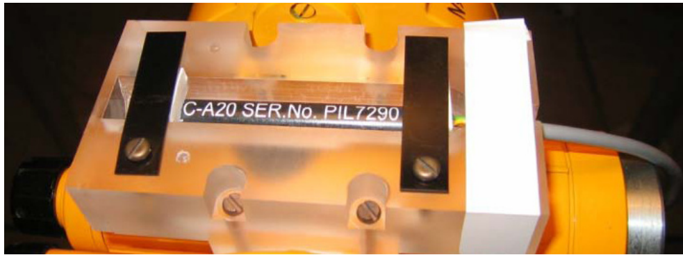
Picture 2 –Pandect sensor mounted in a cradle with nonmagnetic springs for fast replacement or rotation.
