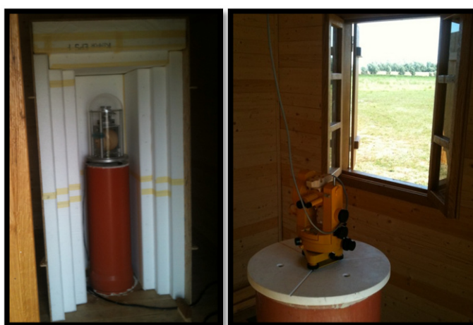
Figure 3 –Left: The dIdD inside the insulation box; Right: The fluxgate theodolite on the absolute pillar.
