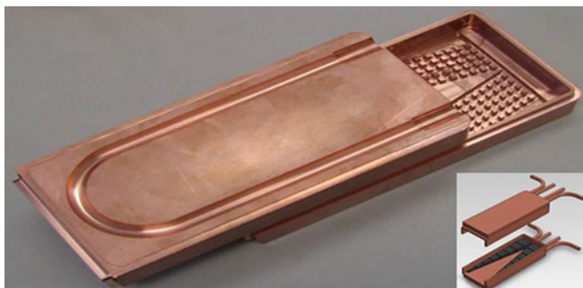
Figure 3. Developmental HOM damper with copper pinbed substrate. Inset shows LOM damper with SiC tiles.
