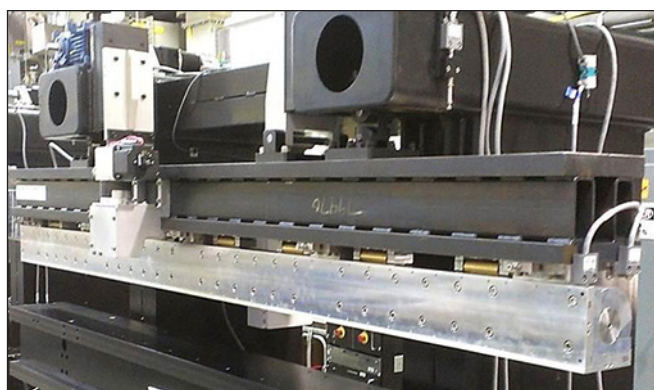
Figure 1. Non-revolving strong-back design. Only the magnet arrays (not shown) and their mounting structures revolve. The revolver drive is located at the mid-point of the arrays to minimize differential torsional deflection of the arrays.
