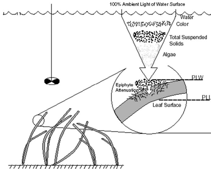
**Figure 3.** Diagram describing the factors influencing the amount of light reaching a seagrass leaf (Batiuk et al., 2000).
