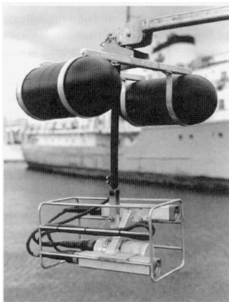
Figure 2: The underwater portion of the Salmon Sizing System showing the video cameras, with flotation device at the top.
