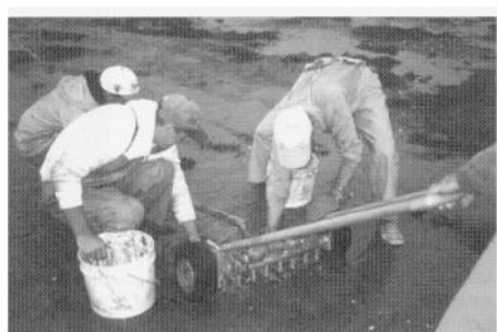
Figure 8: Photo of the hydraulic clam harvester used to collect clams from the beach for the relaying project.
