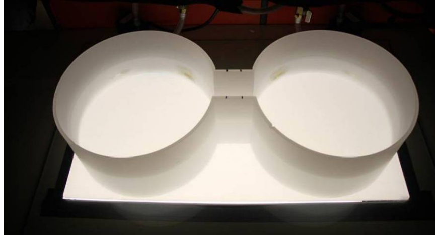
Figure 4. Shuttlebox tank used to test Carmine Shiner ( Notropis percobromus ) temperature preference.
