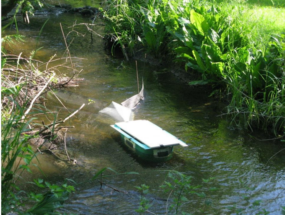
Figure 3A. Typical placement of a trap. In this trap, the tunnel is fine mesh metal screen.
