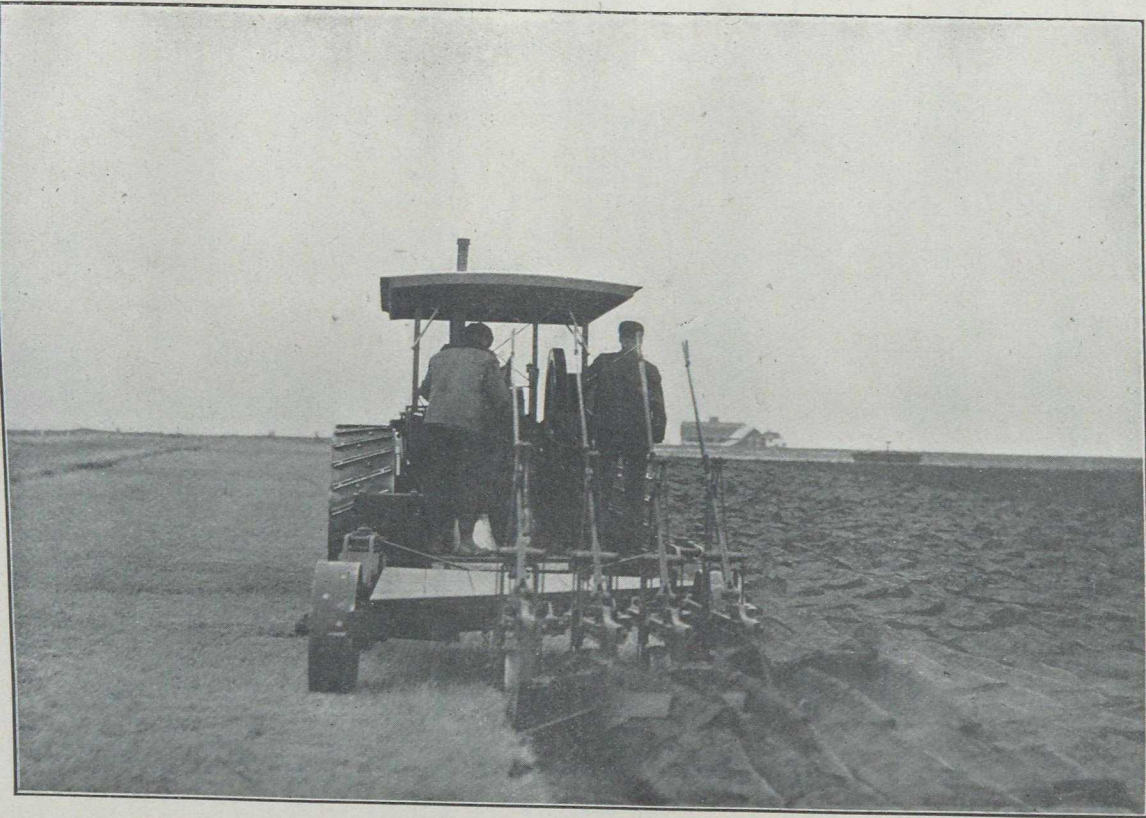
Gasoline Engine at work on the Lethbridge Experimental Farm, pulling four 14-inch ploughs in native prairie soil.
