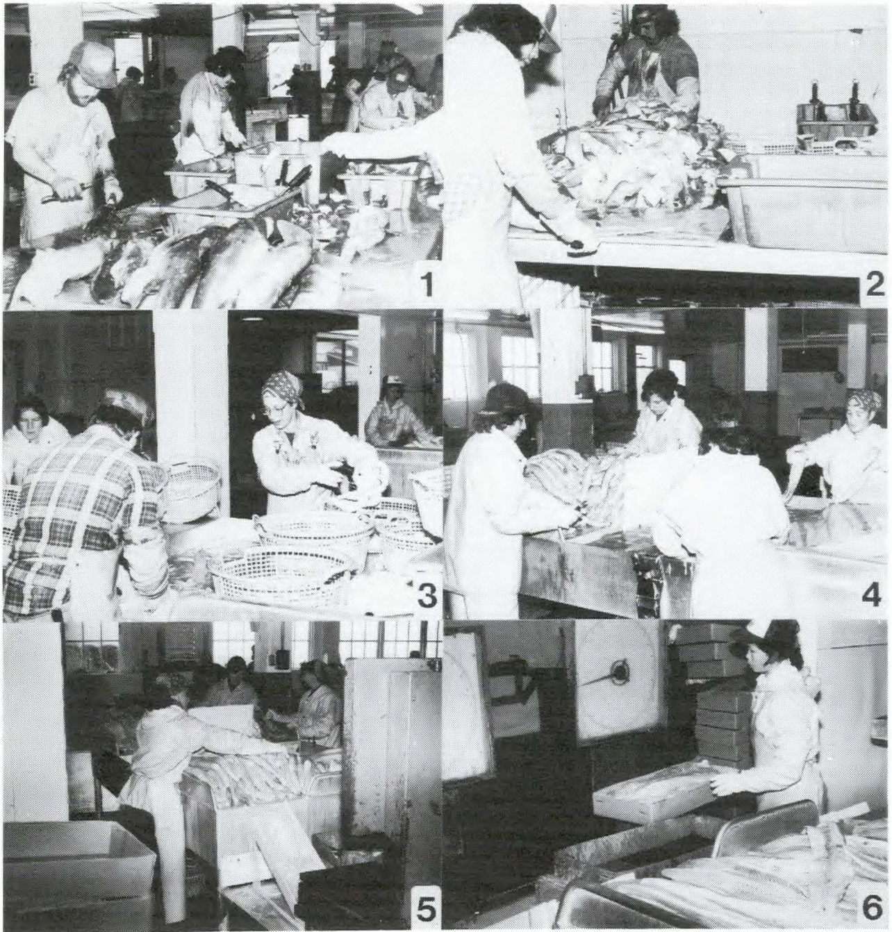
FIG 24. Stages in the processing of spiny dogfish for export of foodfish products to Europe: (1) gutting and skinning operation; (2) filleting of belly-flaps, (3) washing of belly-flaps, (4) washing of backs, (5) individual packaging of backs and (6) boxing of backs for freezing and shipping. Photographs by author, through courtesy of Arrowac Fisheries, Bellingham, Washington.
