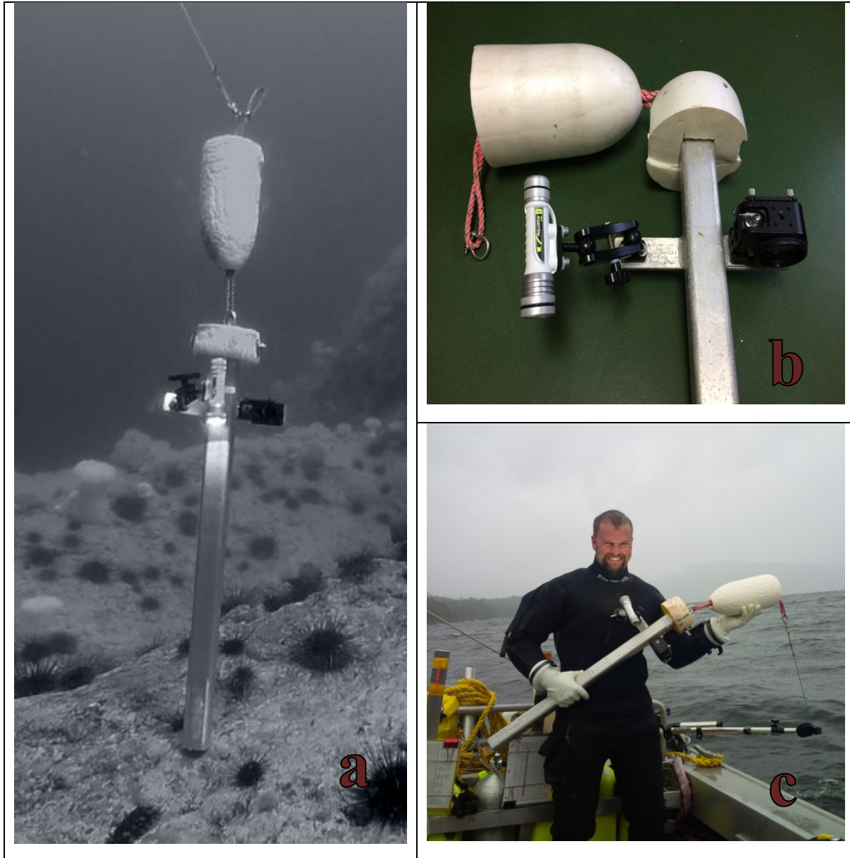
Figure 2. Photos of the drop camera to illustrate the design and scale; (a) the drop camera collecting still images on the seafloor; (b) a close-up of the camera and light housing units and their placement on the monopod; (c) the drop camera attached to a downrigger and ready for deployment in the field.
