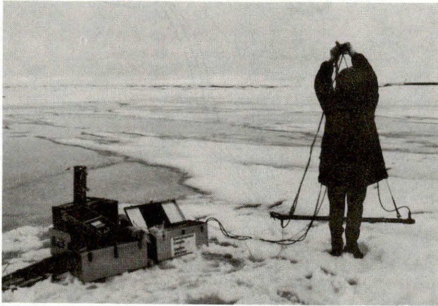
Figure 4. Photograph of H. Chew holding the light sensor support ready for deployment through ice in Balaena Bay, N.W.T. June 4, 1975.
