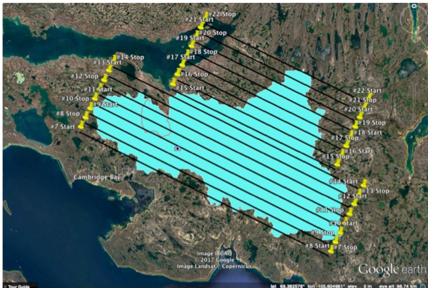
Figure 4: One set of 2017 AVIRIS-ng flightlines (in black) over the CHARS ERA and Greiner watershed (aqua fill colour).
