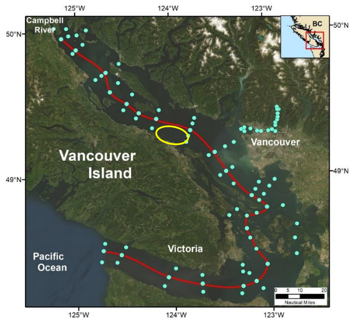
Figure 36-1. Dots show the locations of stations sampled during the water properties surveys. The thalweg is shown as the red line joining the deepest stations along the centerline of the Straits. The yellow ellipse marks the CFMETR data collection area.
