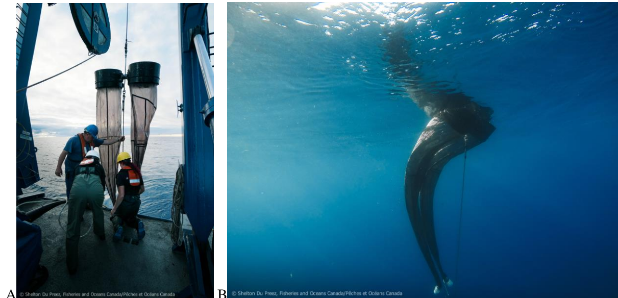
Figure 11. Bongo nets used for oceanographic sampling of the water column A) Being deployed from the aft deck of the E/V Nautilus and B) At the surface of the water column above a seamount (photo credits: Shelton Du Preez, DFO).
