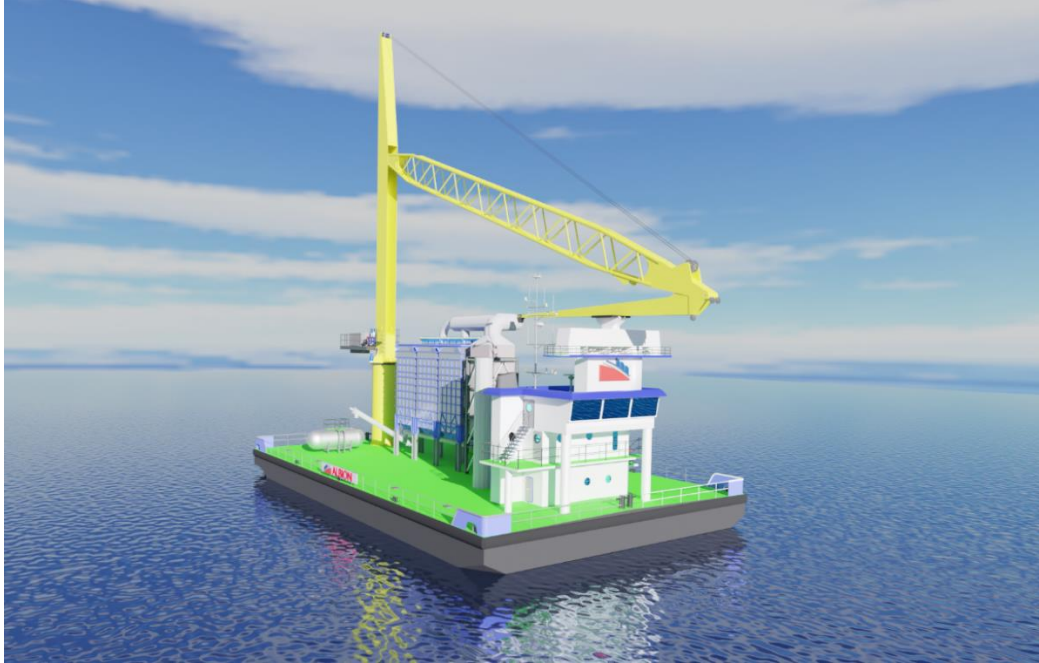
Figure 5. Advanced Air Emission Abatement Floatation Unit
