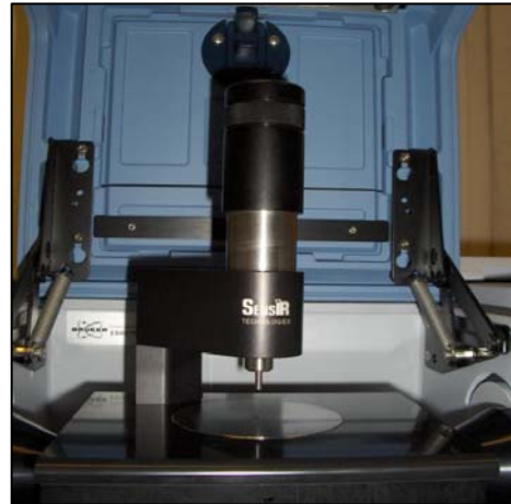
Fig.5: ATR- unit with an attached ATR-Plunger on the bottom side which is pressed on the sample with constant pressure.
